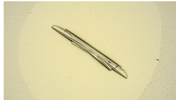
Figure 2: Crystal of Thaumatin. Drop: 20mg/mL protein in water + TbXo4OH 2 mM (observation: + 7 days).
